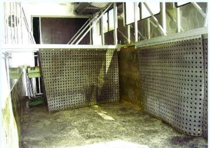
Splitbelt with aeration holes used as dividers in horse floats made by Rivenlee Floats of Armidale. Being light and strong, Splitbelt is used extensively in lining of horse floats.
