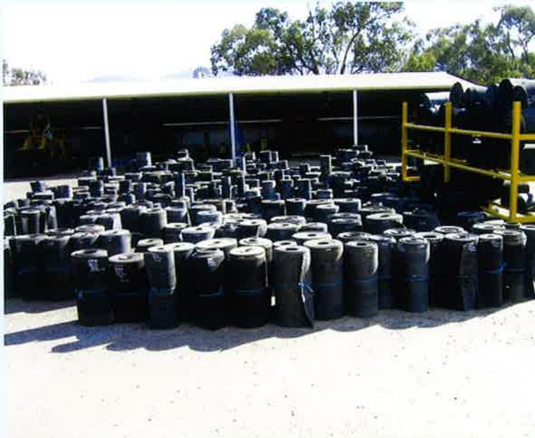
Some of the extensive stocks of Splitbelt in the Andromeda yard. It is sold in rolls as made in the splitting operation
